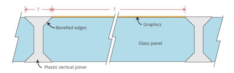
Glass partition graphics are usually installed on the flat surface of the glass only (shown in orange) and not allowed to over run bevelled edges or the plastic joiners between glass panels.
