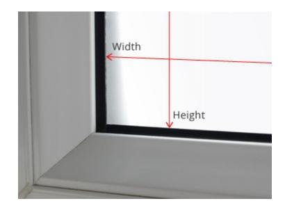
Measure your glass area with a tape measure; taking care to bend the tape into the frame edges to get an accurate reading. You'll find its not possible bend the tape measure all the way into the edge of the seal, so you'll have to estimate were your tape measure will lay, by projecting an imaginary line towards the edge of the rubber seal (see dotted red line)
